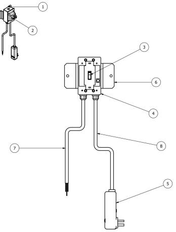
FIGURE 6: SWITCH GFI ASSEMBLY 2016 TO PRESENT
