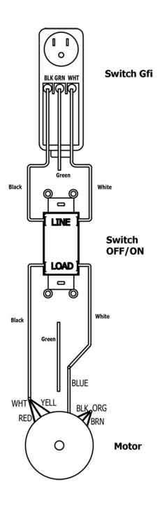
FIGURE 7: WIRING DIAGRAM 2016 TO PRESENT
